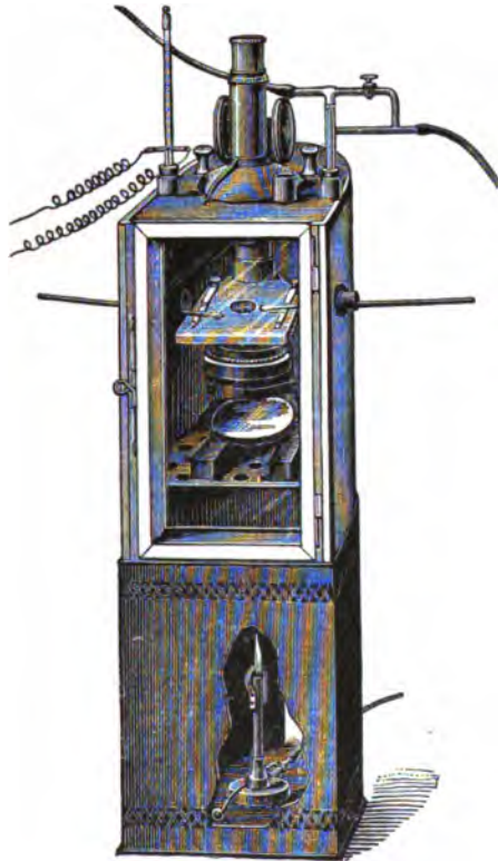
Fig. 33.—Apparatus for keeping objects under microscopic examination at constant temperatures (Nuttall).
